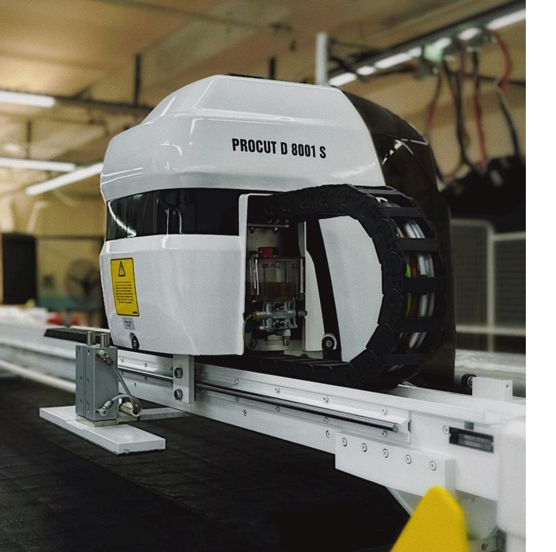
Cutting, sewing, sample sewing, quality control, ironing and packaging processes are carried out within our company. Cutting is performed flawlessly with the BULLMER PROCUT D80015 automatic cutting machine.
